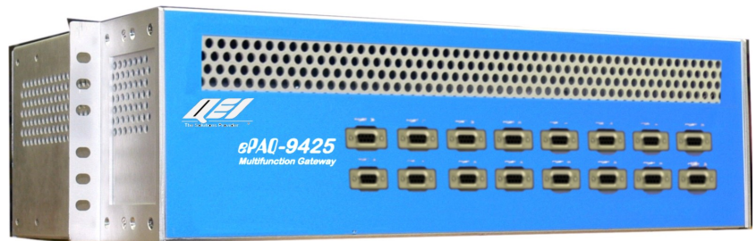
ePAQ-9425 Rear Panel DB-9 Serial Connection.
